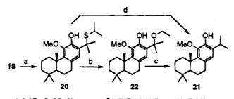
a) i. +Pr<sub>2</sub>S, SO<sub>2</sub>Cl<sub>2</sub>, pyr, -40 °C ii. Et<sub>3</sub>N; b) Raney Ni, EtOH, reflux 1 h, 51%; c) H<sub>2</sub>, Pd, acid, 100%; d) Raney Ni, EtOH, reflux 1 h, 61% from 18.
